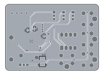
Figure 6: AAT2842 Evaluation Board Bottom Layer.
