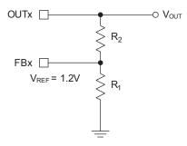
Figure 2: Selection of External Resistors.
