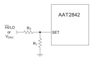
Figure 4: Brightness Control Using Either BSET or FSET Resistor Pin.
