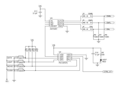
Figure 8: MCU and I/O Expander Section Schematic.
