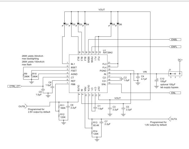
Figure 7: AAT2842 Section Schematic.
