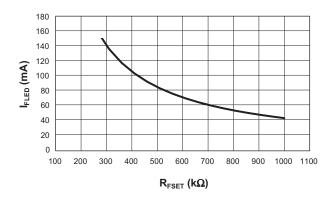
Figure 3: Maximum Flash Current vs. R<sub>FSET</sub>.
