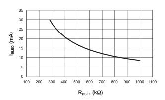
Figure 2: Maximum LED Current vs R<sub>BSET</sub>.
